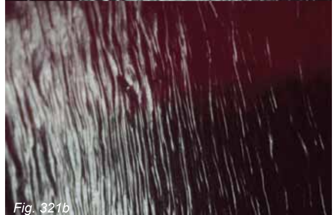
Fig. 321a-b Details of the striae on the rough of synthetic spinel indicates that the spinels were pulled in the process when they were synthesized from a flux. Rings perpendicular to it also indicate that they were rotated.
