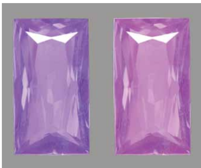
Fig. 323 Color-changing synthetic spinels produced by flux (pulled method), with color-change from violet (in daylight) to purplish-pink (in incandescent light). Approximately 1ct, cut by GRS from the rough.
