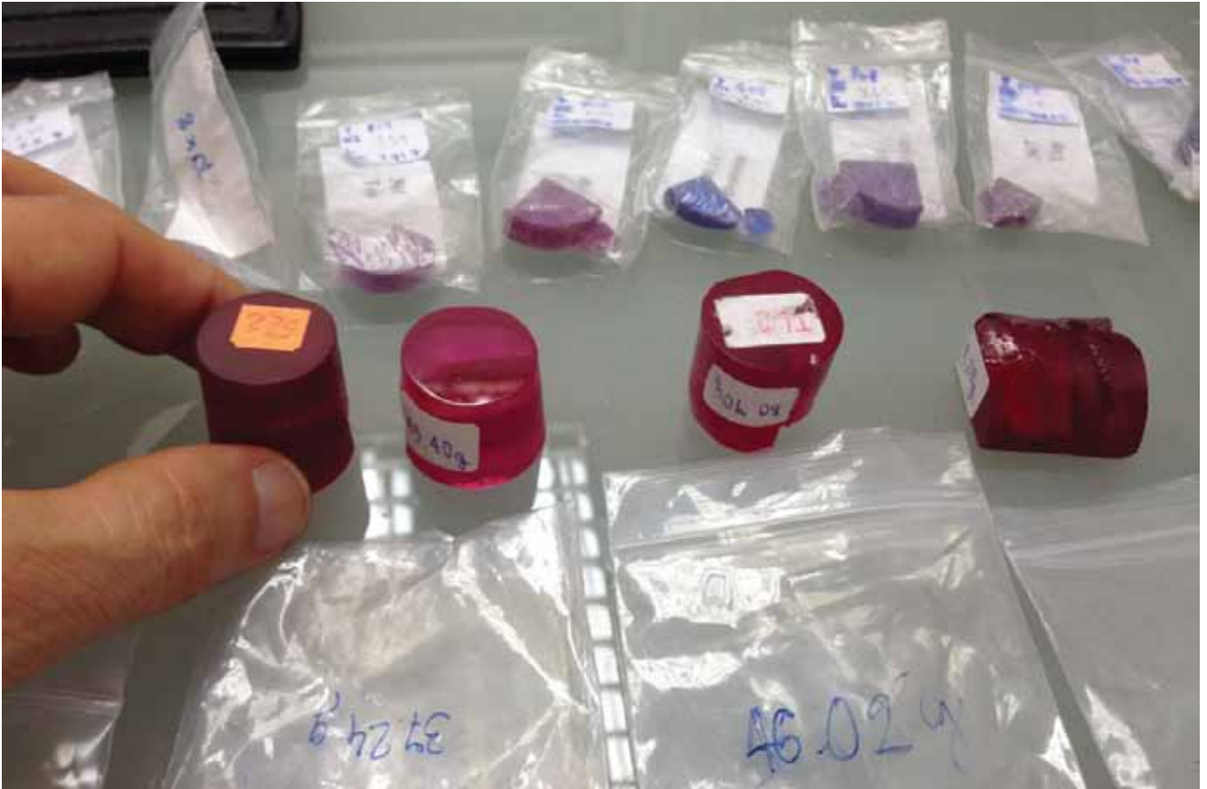
Fig. 320 Spinel commercially produced by the pulled method from flux. Note the approximate 5cm diameter of the cylinders and the different color varieties. The rough is about 250ct in size. Photo by AP at Tairus, Bangkok.
