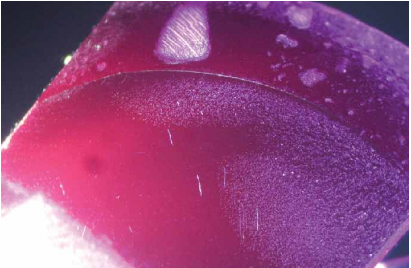
Fig. 327 Inclusion in a rough synthetic spinel of pinkish-red color. Myriads of pinpoint bubbles may be seen in concentrated areas.
