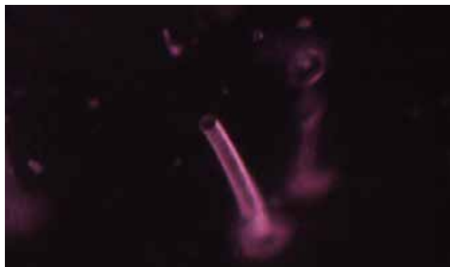
Fig. 319 Tube inclusion in synthetic spinel of purple color. The tube shows a screw-like mark at the surface indicating that the spinel was produced by turning from a flux.
