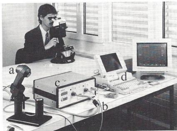
The four (a-d) main pieces of equipment used to color grade diamonds by means of computer-based multichannel spectroscopy.
