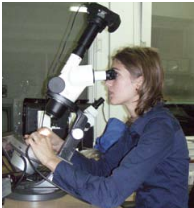
Fig. J29. One of the authors (FP) on the GRS micro-photography station used for this study. It included a Canon EOS 350d Digital Camera, mounted to a trinocular Zeiss Stemi 2000-C microscope and a cold light Eickhorst base. The Digital camera system is controlled by a Mac notebook.
