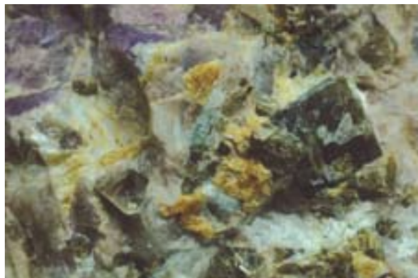
Fig. J61 Typical pegmatite with johachidolite (yellow), apatite (green), scapolite (white), orthoclase (gray), phlogopite (brown) and hackmanite (purple). A negative Eu anomaly is found in johachidolite and apatite (See Fig. J73 and J74).
