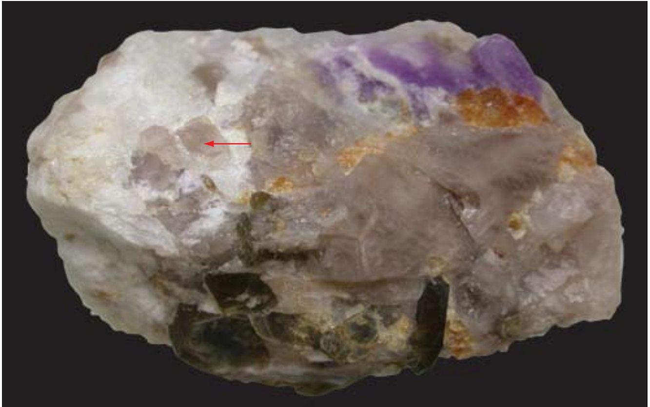
Fig. J67. Rock specimen with scapolite on the left and orthoclase on the right, as well as hackmanite (purple), phlogopite and johachidolite (orange). Orthoclase is formed prior to scapolite and can be found as inclusions in scapolite (arrow). GRS-Ref 5630.
