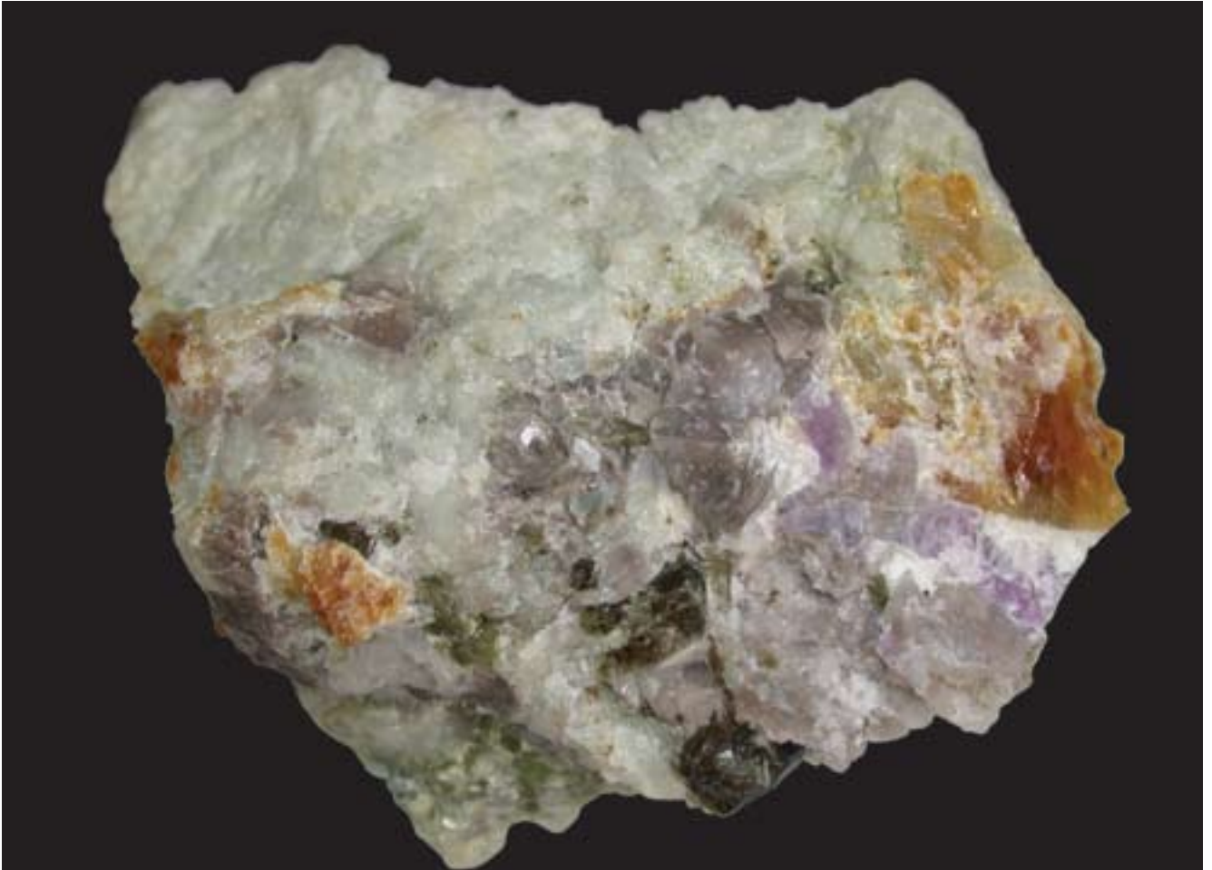
Fig. J44. Mineralogical composition of pegmatite: Johachidolite (orange), scapolite (white), orthoclase (gray), phlogopite (brown) and apatite (green). Quartz and minerals of the beryl group are absent. The sample is 10 cm large. Scapolite is most abundant in the rock.
