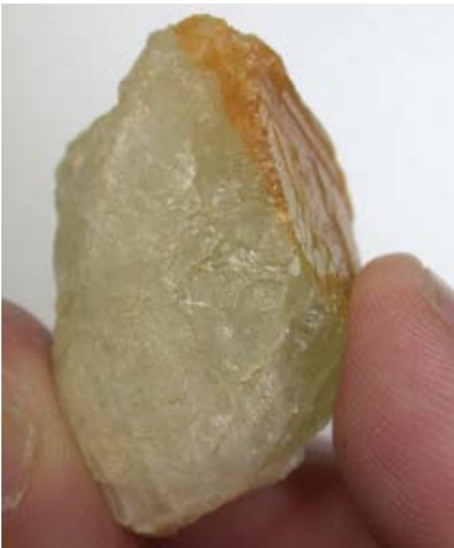
Fig. J 54. Example of a large johachidolite rough of 94 ct. Three colors are found in the rough, including colorless, light green and yellow-orange. The yellow-orange color is confined to the outer rim of the rough fragment, which represents the latest growth phase. The coloration of johachidolite is related to a drastic change in formation conditions, which occurred along a distinct phase of growth along a sharp zone in the crystal. Sample GRS-Ref 5649.
