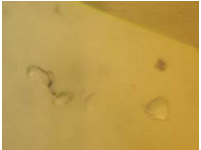
Fig. J33. Johachidolite with a series of transparent and round solid inclusions (60x magnification) found in a faceted sample of yellow color (0.72 ct). They are rarely found in the otherwise clean stones. GRS-Ref 5937.
