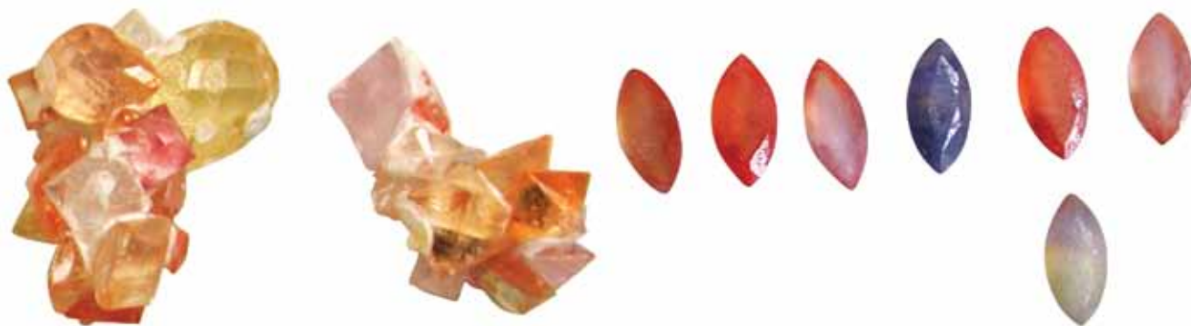
Fig. A3 Different colors produced by the new treatment (including pink, yellow, orange, and blue) are sorted for this report. Sapphires of different colors are accidentally clustered together by the melting of minerals other than sapphire during heat treatment with Beryllium. Only a small portion of the sapphires showed this accidental cluster. Note: Different colors are produced in the same heating runs.
