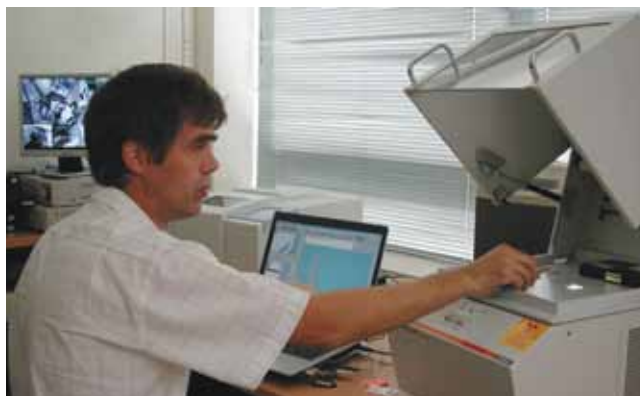
Fig. A18a Example of an ED-XRF Spectrometer used for chemical testing of corundum at GRS. A sample is positioned at the window above a X-ray generator by Dr. A. Peretti.
