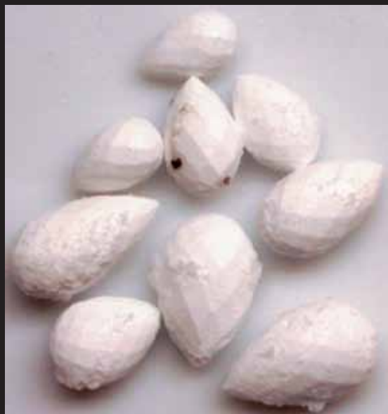
Fig. A11 Macrophotograph of glass-aggregate formed by the melting of non-sapphire materials during heat-treatment with Beryllium.
