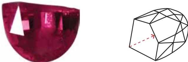
Fig. B38 Microphotograph of GRS 29 (synthetic ruby) Fig. B39 Drawing of GRS 29. Analysis was performed with 21 spots along the broken line (crater diameter: 80 \mu\text{m} )
