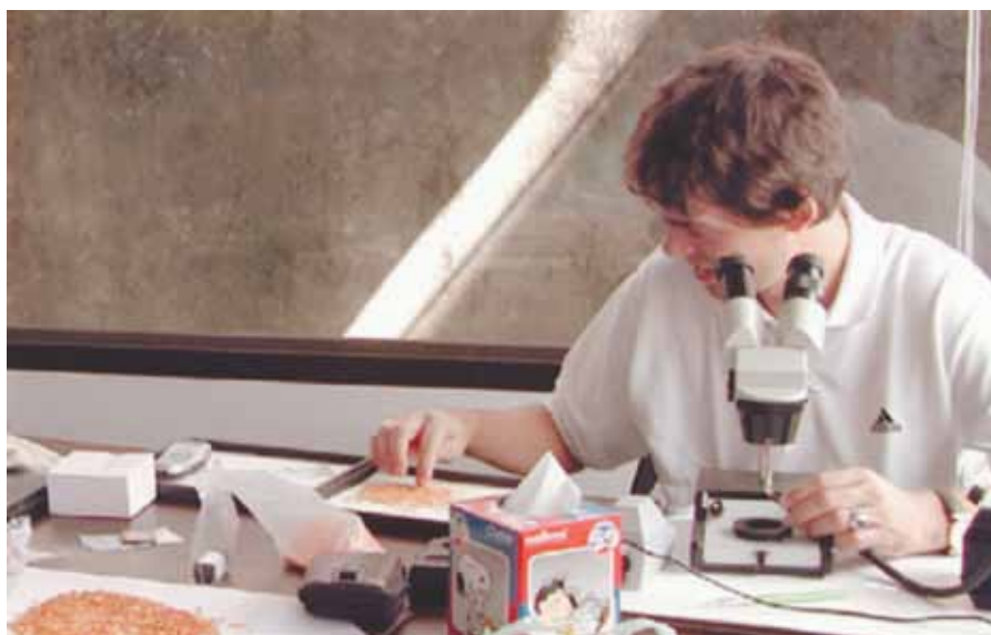
Fig. A2 Dr. A. Peretti selects samples (Chantaburi, 14th December, 2001) heated-treated with Beryllium , sorts the different colors of produced sapphires and non-sapphire crystals (as shown in Fig. A8) and then carries out gemological tests (using a portable microscope, portable fiber-optic light source of 100 watt power, Geiger counter, Dichroscope, Polariscope, Refractometer and UV-lamp). Later, in Bangkok, he continues the tests using a vertical trinocular microscope (65x magnification) and a horizontal microscope from Eickhorst with an immersion unit (GEMMASTER SUPERSCOPE).
