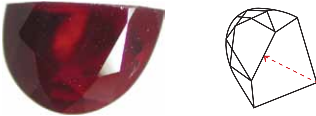
Fig. B35 Microphotograph of GRS 27 (synthetic ruby) Fig. B36 Drawing of GRS 27. Analysis was performed with 16 spots along the broken line (crater diameter: 80 \mu\text{m} )
