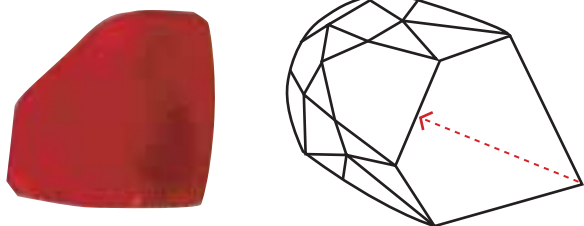
Fig. B27 Microphotograph of GRS 25 (synthetic ruby) Fig. B28 Drawing of GRS 25. Analysis was performed with 18 spots along the broken line. (Crater diameter: 80 \mu\text{m} )
