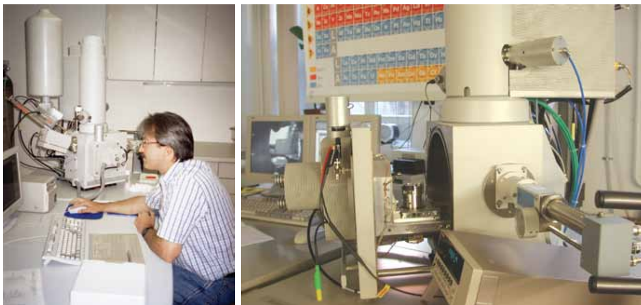
Fig. A7 An example of a SEM-EDS recently used for research is shown from the University of Fribourg, Earth Science Department, Switzerland. On the left: Prof. B. Grobety operating the SEM (FEI XL 30 Sirion FEG). To the right details of the SEM: An opened sample chambre, surrounded by a variety of detectors, such as Secondary Electron Detector (SE), Backscattered Electron Detector (BSE) and an X-Ray Detector (EDS) with a Polymer Window (S-UTW), for microchemical analysis.
