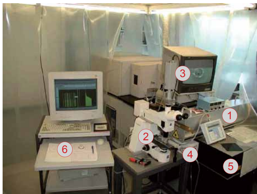
Fig. A32 Laser Ablation Mass Spectrometry (LA-ICP-MS) at the Laboratory for Inorganic Chemistry, SFIT ZH, Switzerland (Prof. D. Günther)
