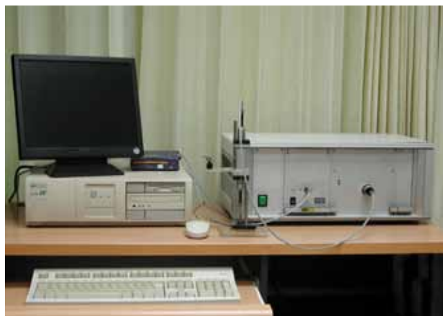
Fig. A25 The GRS UV-VIS-NIR multi-channel spectrometer used for recording the absorption spectra of the gemstones. A special measuring chamber set-up (Center of picture) enables the collection of non-polarized, or polarized absorption spectra, between 290nm (UV) and 1024nm (NIR) on rough or faceted gemstones in all different crystallographic directions within milliseconds.
