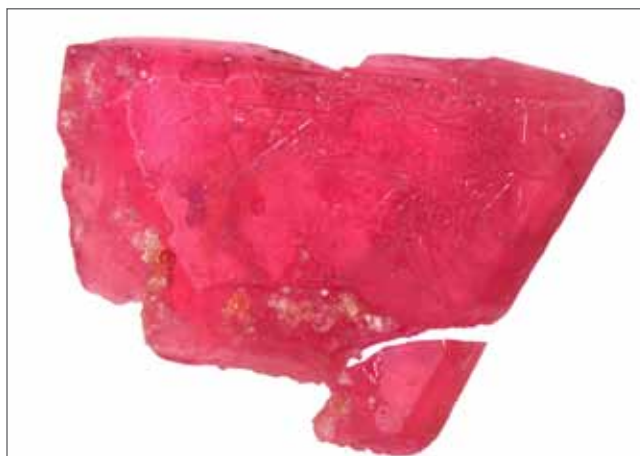
Fig. P5 Pezzottaite tabular crystal of 29.41ct and a broken part of it (lower right), which served as the sample used for the Swiss team's detailed chemical and crystallographic investigations. The lower right piece parted in 3 different fragments which are currently at the University of Berne (see Box 6), the University of Fribourg, and the SFIT (Switzerland). The remaining motherpiece of 29.41 ct is in the GRS collection.
