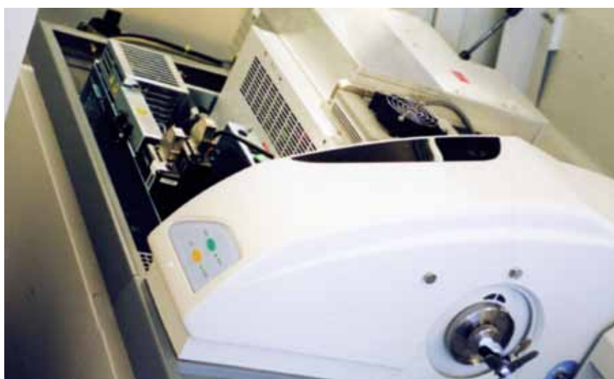
Fig. 38 Detailed image of the microscope, sample chamber (above) and Mass-spectrometer (below) used for LA-ICP-MS analysis. Applications - See: Guillon M. and Günther, D.(2001): 'Quasi "non-destructive" Laser Ablation-Inductively Coupled Plasma-Mass Spectrometry Fingerprinting of Sapphires. Spectrochimica Acta Part B, 56, p 1219-1231.
