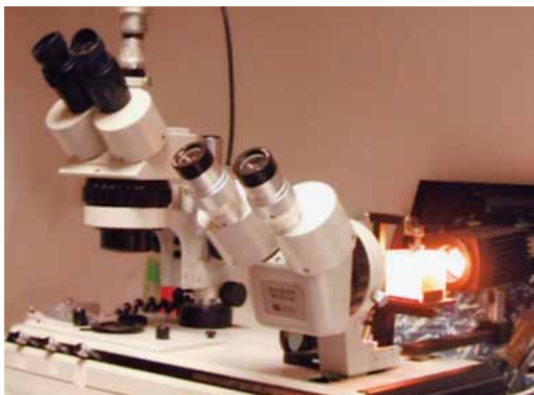
Fig. 2 Dr. A. Peretti selects samples (Chantaburi, 14th December, 2001) enhanced with the new method, sorts the different colors of produced sapphires and non-sapphire crystals (as shown in Fig. 8) and then carries out gemological tests (using a portable microscope, portable fiber-optic light source of 100 watt power, Geiger counter, Dichroscope, Polariscope, Refractometer and UV-lamp). Later, in Bangkok, he continues the tests using a vertical trinocular microscope (65x magnification) and a horizontal microscope from Eickhorst with an immersion unit (GEMMASTER SUPERSCOPE).
