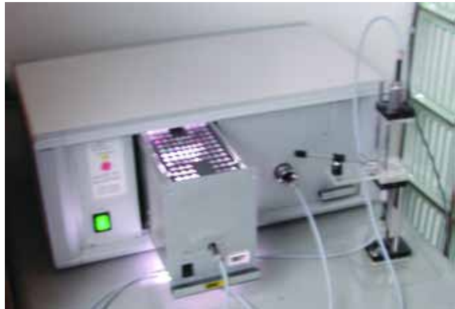
Fig. 21 The GRS UV-VIS-NIR multi-channel spectrometer used for recording the absorption spectra of the gemstones. A special measuring chamber set-up (To right of picture) enables the collection of non-polarized, or polarized absorption spectra, between 290nm (UV) and 1024nm (NIR) on rough or faceted gemstones in all different crystallographic directions.
