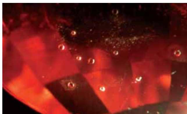
Fig. 67 Sample No.GRS 782 Natural Orange-red Sapphire from Songea (Tanzania) enhanced with the new E(IM)-method. Craters from scattered LA-ICP-MS Testing.
