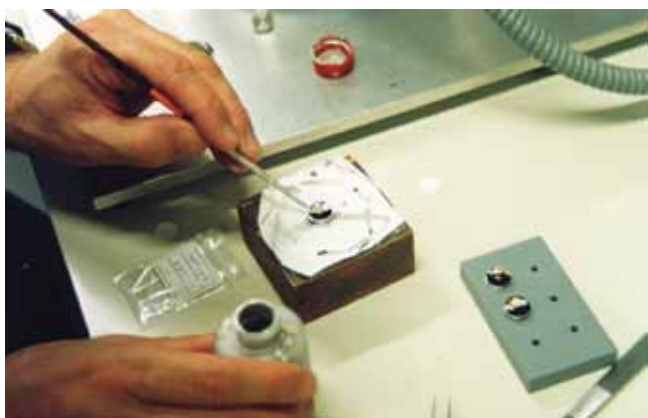
Fig. 9. Dr. A. Peretti mounts the Chrysoberyl samples for SEM-EDS analysis in February 2002 at the University of Basel (Switzerland).
