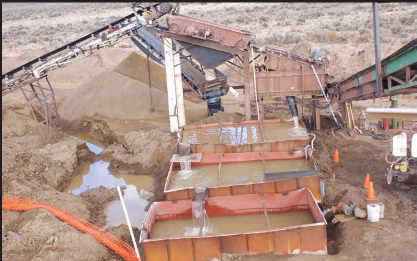
Fig. An14B The washing plant at the Dust Devil Mining in Oregon (USA) is shown. Only water is utilized and environmental standards are cared for.
