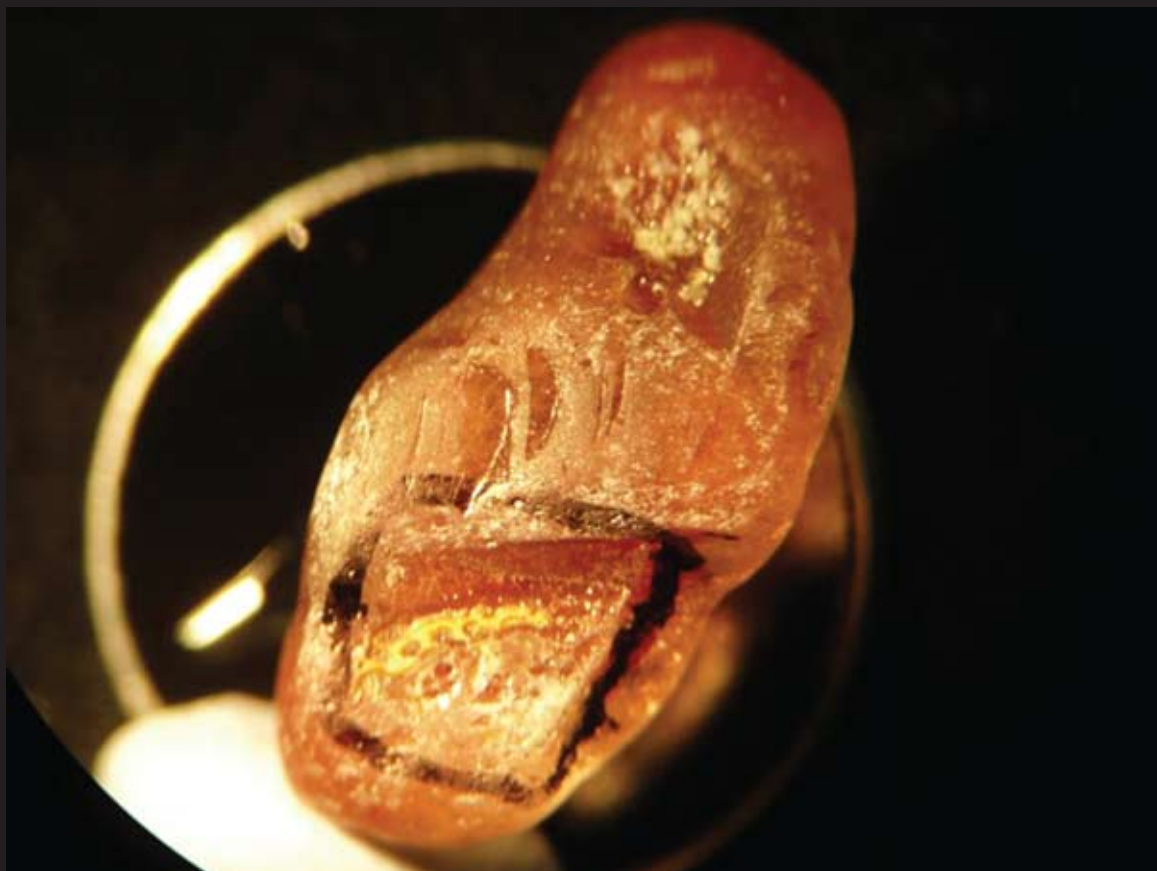
Fig. An80 Image of a sample from the old mine in Tibet (Expedition 2008, Bainang) with measuring positions and enlarged (See Fig. An79). Areas studied in detail by SEM-EDX are indicated.
