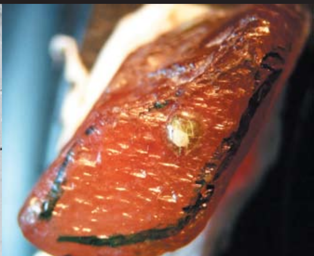
Fig. An60A Diffusion-treated andesine from Shenzhen with a glassy residue on its surface. Length of crystal is 15mm.
