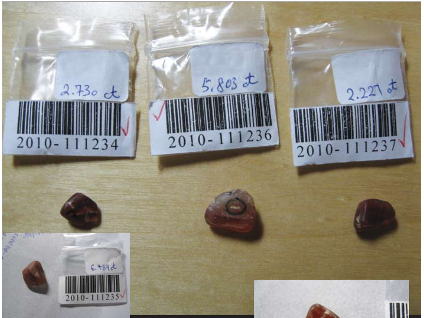
Fig. An18 The samples of group A(2) (See Tab.An01) are shown. Samples appeared water-worn or tumbled. Cracks and cavities were filled with minerals and glassy residues. These fissures and cavities were analyzed in more details (See Fig. An90, An94-95, An97, Tab. An02, Tab. An04, Tab. An07).
