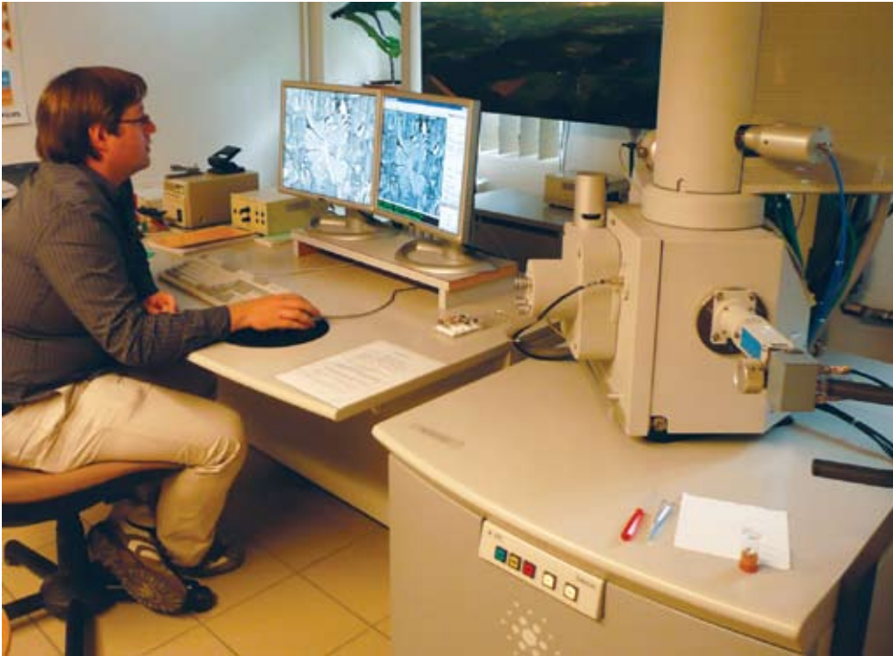
Fig. An58 Portrait of the laboratory (Group: Prof. B. Grob ty) of the University of Fribourg equipped with a FEI XL30 Sirion FEG scanning electron microscope. The working scene shows one of the author's (MM) discovery of the delicate copper-bearing dendrites on the surface of a diffusion-treated andesine with a SE detector used for highly detailed and resolved images (See also Fig. An59).
