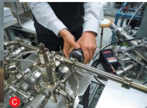
Fig. An99 Extraction system used for the determination of Ar* concentrations in natural and diffusion-treated copper-bearing andesine.
