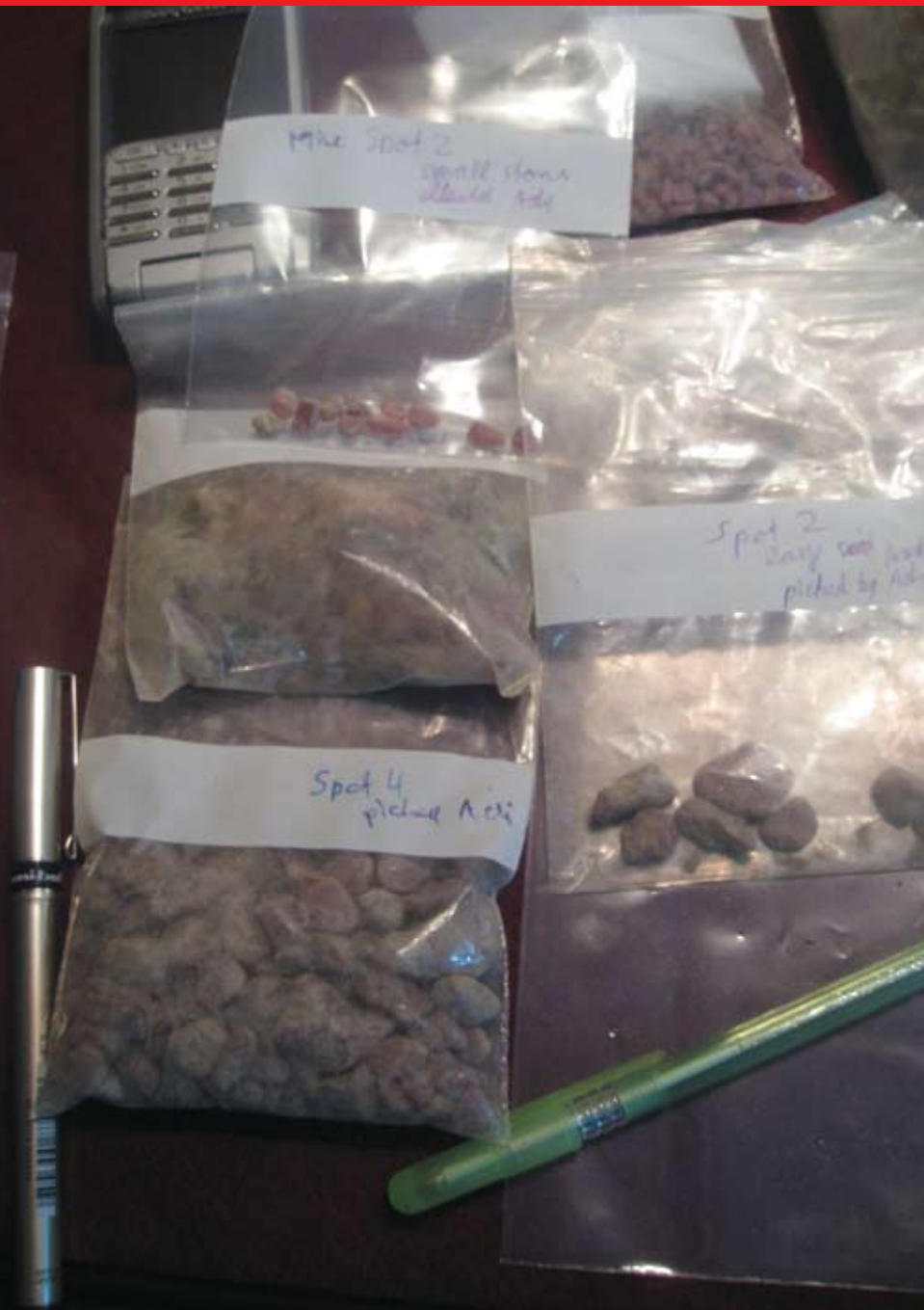
Fig. An23 These samples were collected from 4 mining spots all in disturbed layers at the bottom of several meter deep open pits. From these materials we polished a set of samples that are shown. These included materials with concentric color zoning (green core and red rim, with red color zoning and with alternating red and green color zoning). Further analyses of this material confirmed the field observation that the mine was salted. The materials were found to be natural untreated materials from other collection points in Tibet. Further samples See Fig. An24-27.
