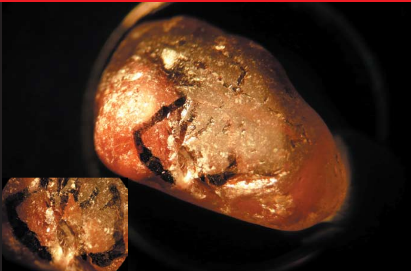
Fig. An75 Image of the copper-bearing andesine analyzed with SEM-EDX containing glassy residues in cavities.
