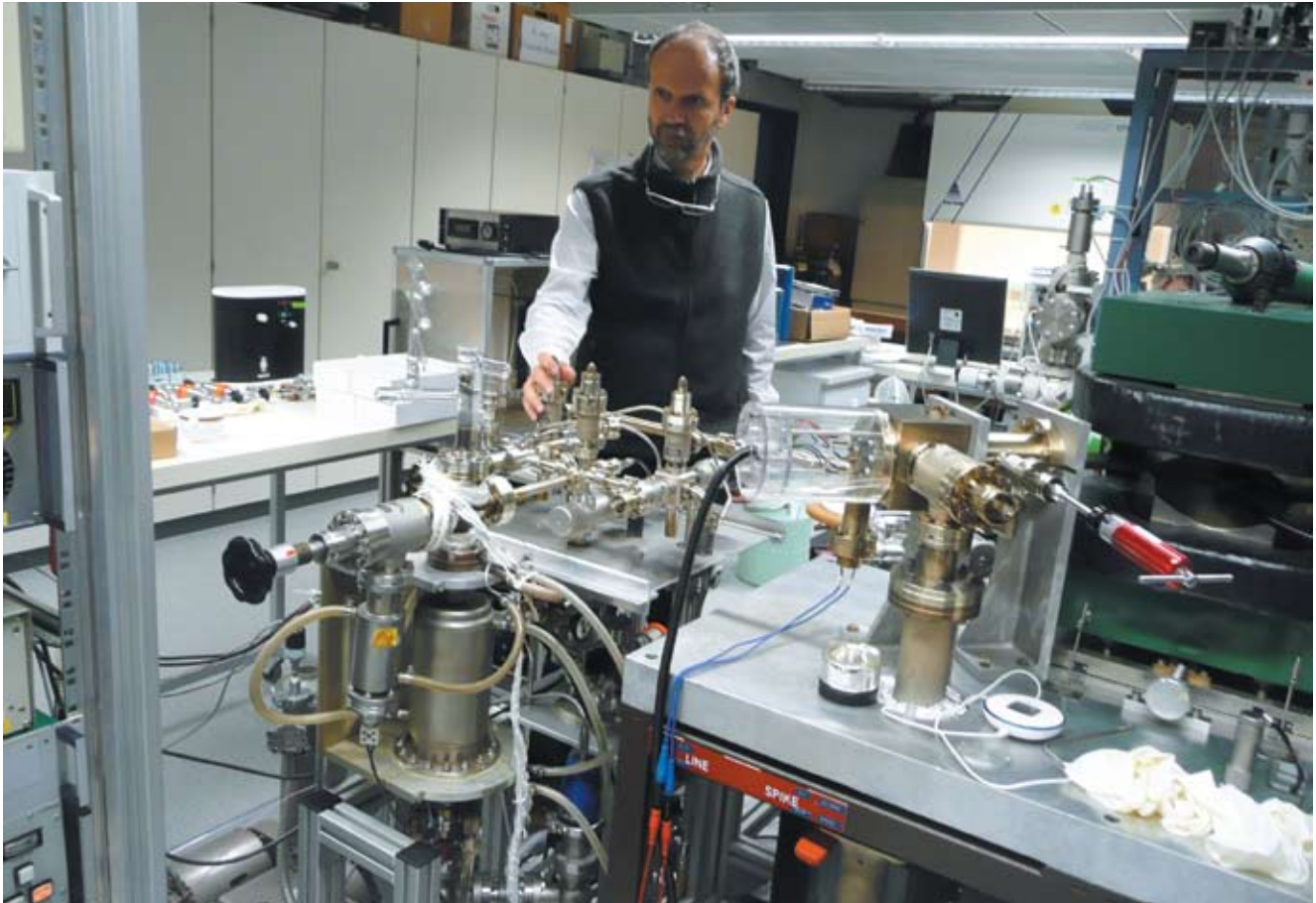
Fig. An98 Mass spectrometer used for the determination of Ar* concentrations in natural and diffusion-treated Copper-bearing andesine
