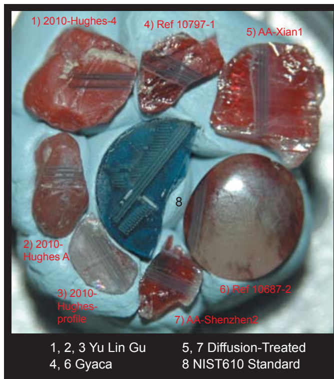
Fig. An103 The samples shown in the figure were analyzed by fs-LA-MC-ICP-MS in scanning mode. The integration time was 30 seconds, which corresponds to 600 \mu\text{m} sections on the sample. In the plots, the open symbols are for the different sections of the 3 runs. The averages in the plots (closed squares) correspond to the average over the 3 runs for the same section.
