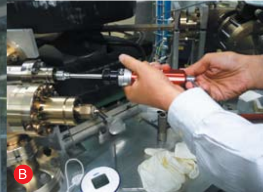
Fig. An98 Mass spectrometer used for the determination of Ar* concentrations in natural and diffusion-treated Copper-bearing andesine
