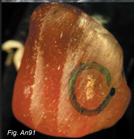
Fig. An90A-B A 5 \mu\text{m} large silver platelet was found on the surface of this Tibetan andesine (Fig. An91) from the expedition in 2008 (Lit. An01). The samples were hand-collected from the mine and supplied to GRS in 2011 (Ref-No. 2011-111236, Fig. An18). BSE-image is inserted (Fig. An90B) and EDX spectrum of the particle identifies it as native silver (measurement includes matrix).
