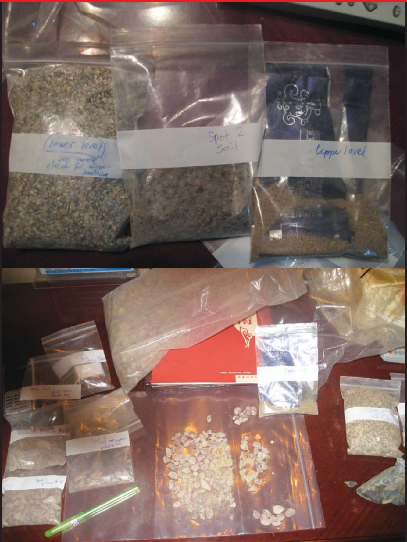
Fig. An22 The upper picture shows the different sizes found in the alluvial deposit with silt and sand sizes collected from layers with sedimentary structures. No copper-bearing andesine was found in these lots. Large amount of 5-20mm sized copper-bearing andesine samples were collected and sorted according to the spot of findings. Hand-collected samples are in the bags on the lower left. Other samples were taken from the mined lots that were present in a container at the production site (Expedition details See page 06-13).
