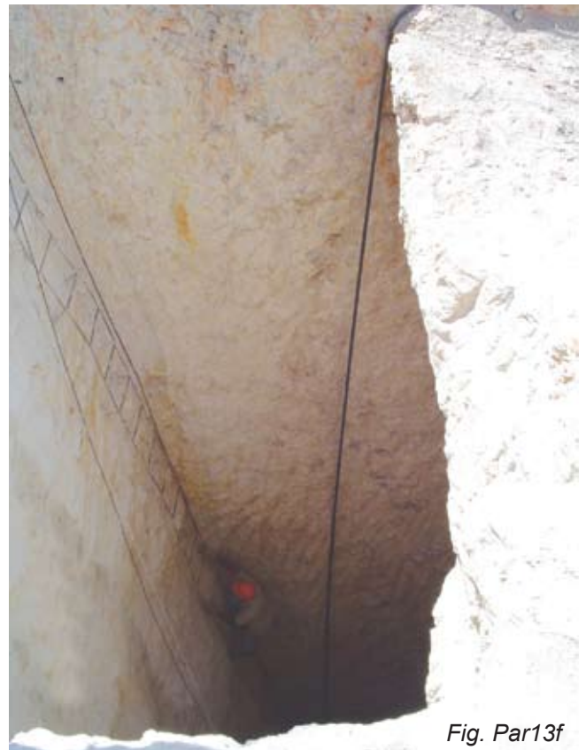
Fig. Par13c-f A view into the underground mining of "Paraiba"-tourmalines in the Heitor shaft (Batalha mining area, Paraiba, Brazil). The vertical shafts are driven to a depth of 40m in soft "kaolinized" pegmatites (Fig. Par13e-f). Underground tunnels are partially collapsed (Fig. Par13d). Picture Markus Paul Wild. P. Wild Archive.
