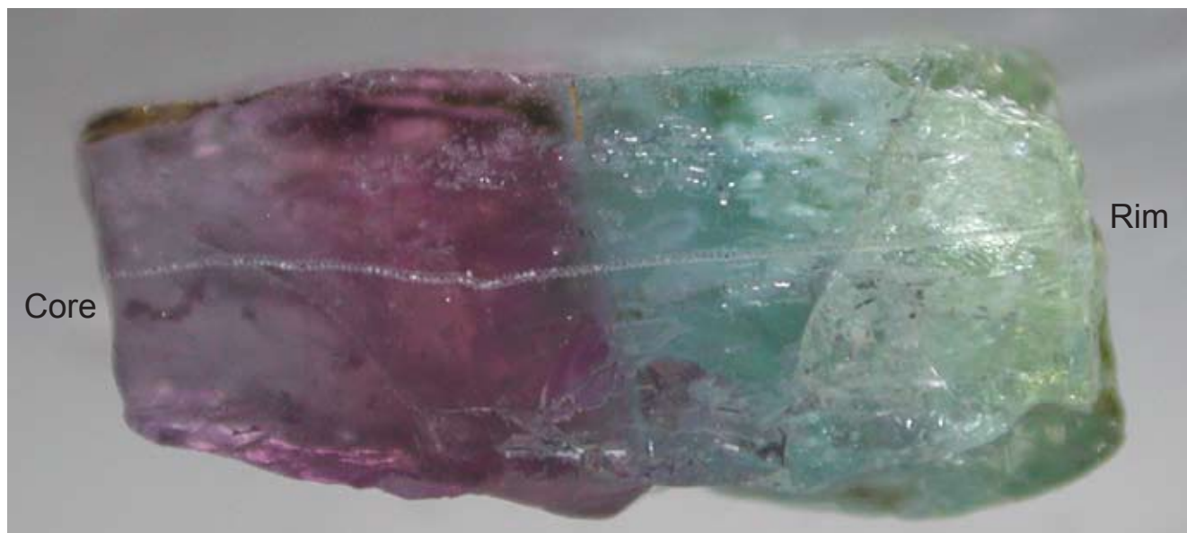
Fig. Par77 Photograph of a multi-colored tourmaline from Mozambique, Sample No. GRS-Ref3134. Violet, greenish-blue and green color zoning is present (from core to rim). Laser ablation craters are visible (size 60 micrometers). Chemical analysis profiles see Fig. Par78a-f.
