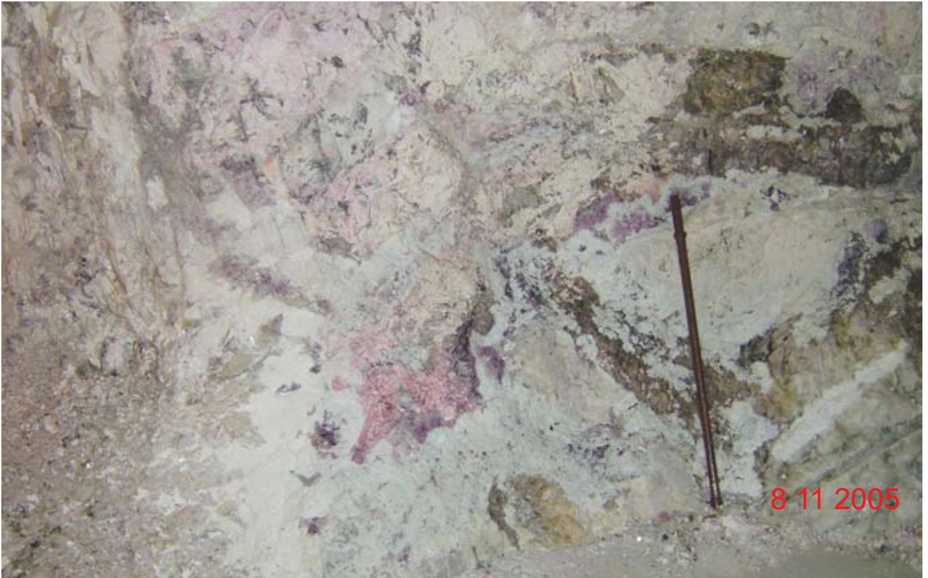
Fig. Par18a A view into the underground rock formations containing pegmatite materials with copper-bearing tourmalines, albite (white) and quartz (grey) in the "Heitor"-mine (Purple = tourmaline and lepidolite). Picture P. Wild Archive.
