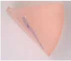
Fig. E14 Microphotograph of GRS 12 (synthetic pink sapphire) Fig. E15 Drawing of GRS 12. Analysis was performed with 40 spots along the broken line (crater diameter: 80 \mu\text{m} )
