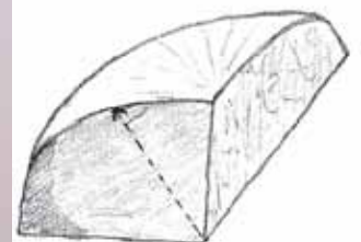
Fig. E23 Microphotograph of GRS 18 (synthetic deep orange sapphire) Fig. E24 Drawing of GRS 18. Analysis was performed with 35 spots along the broken line (crater diameter: 80 \mu\text{m} )
