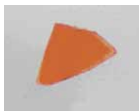
Fig. E44 Microphotograph of GRS 30 (synthetic orange sapphire, Beryllium-treated sample GRS 29) Fig. E45 Drawing of GRS 30. Analysis was performed with 20 spots along the broken line (crater diameter: 80 μm)
