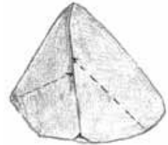
Fig. E41 Microphotograph of GRS 28 (synthetic orange sapphire, Beryllium-treated sample GRS 27) Fig. E42 Drawing of GRS 28. Analysis was performed along the two broken lines (crater diameter: 80 μm) Side 1: 23 pits; Side 2: 15 pits
