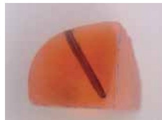
Fig. E23 Microphotograph of GRS 18 (synthetic deep orange sapphire) Fig. E24 Drawing of GRS 18. Analysis was performed with 35 spots along the broken line (crater diameter: 80 \mu\text{m} )
