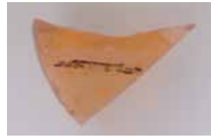
Fig. E20 Microphotograph of GRS 13 (synthetic pink sapphire) Fig. E21 Drawing of GRS 13. Analysis was performed with 33 spots along the broken line (crater diameter: 80 \mu\text{m} )
