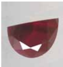
Fig. E38 Microphotograph of GRS 29 (synthetic ruby) Fig. E39 Drawing of GRS 29. Analysis was performed with 21 spots along the broken line (crater diameter: 80 μm)
