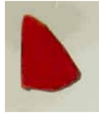
Fig. E41 Microphotograph of GRS 28 (synthetic orange sapphire, Beryllium-treated sample GRS 27) Fig. E42 Drawing of GRS 28. Analysis was performed along the two broken lines (crater diameter: 80 μm) Side 1: 23 pits; Side 2: 15 pits
