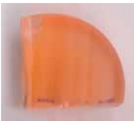
Fig. E17 Microphotograph of GRS 17 (synthetic deep orange sapphire) Fig. E18 Drawing of GRS 17. Analysis was performed with 80 spots along the broken line (crater diameter: 80 \mu\text{m} )
