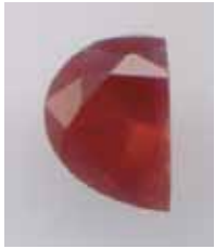
Fig. E35 Microphotograph of GRS 27 (synthetic ruby) Fig. E36 Drawing of GRS 27. Analysis was performed with 16 spots along the broken line (crater diameter: 80 μm)
